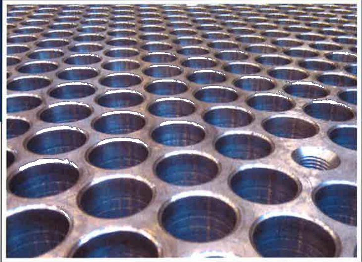
Tubesheet Face Showing Grooved & Rolled Tubes
